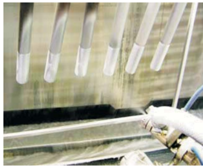
Picture 6. Delta-MKS rack coating of hexagon bolts for wind energy plants Picture: EOT
