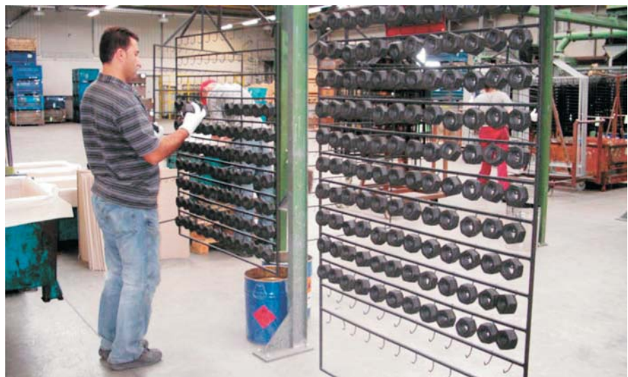
Figure 5. Delta-MKS rack coating of nuts for wind energy plants, picture: EOT
