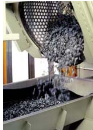
Figure 2: Freshly coated bolts being tipped from the cage onto the baking conveyor in bulk coating
