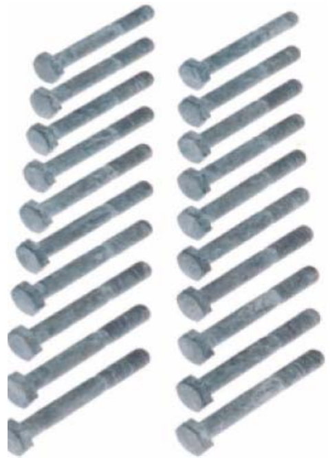
Figure 2. High-performance corrosion protection ›Delta-Protekt‹: Test-bolts, coated with ›Delta-Protekt KL 100‹ and ›Delta-Protekt VH 300‹ after 1000 hours of testing according to SST DIN 50021
