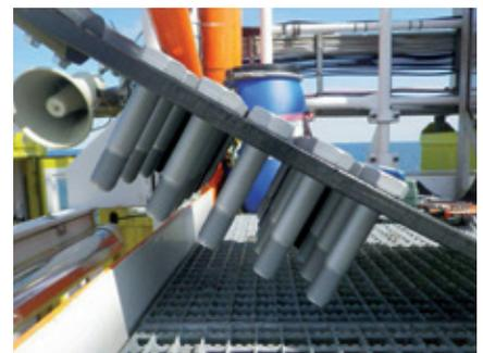
*Moving diverse M24 bolt specimens to the FINO platform in the Baltic Sea.*
