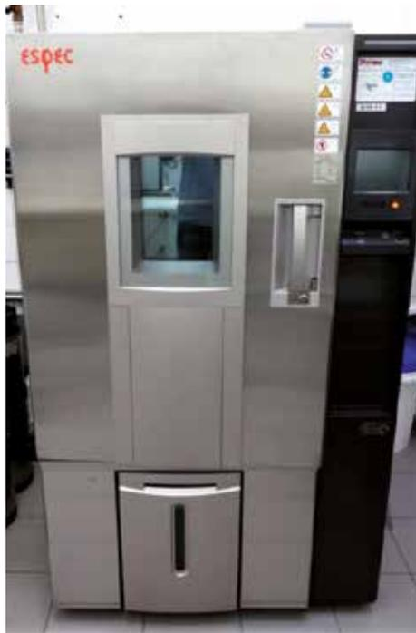
Test chamber for the climatic extremes test (-40/+80°C)
