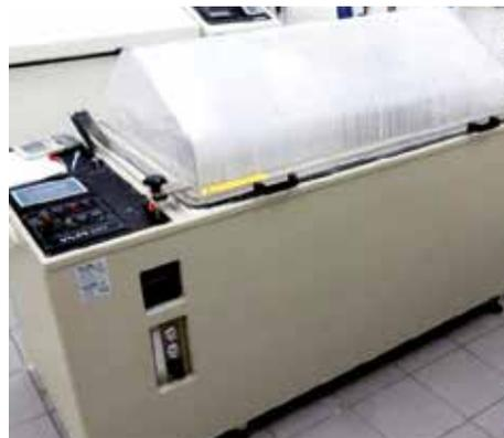
Test chamber for the salt spray test ISO9227 NSS
