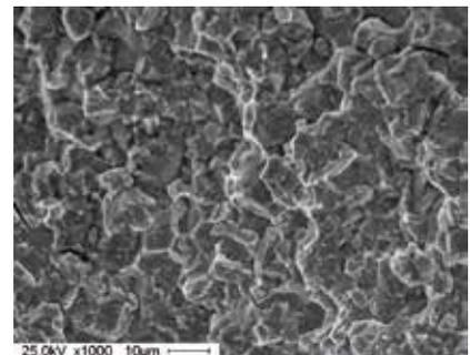
Ruptured surface near to the start of the rupture: inter-crystalline forced rupture showing characteristics of hydrogen embrittlement
