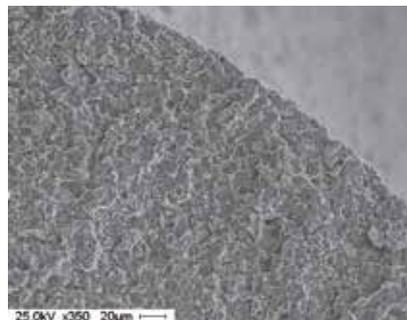
Rupture's starting area, curved forced rupture originating from the surface
