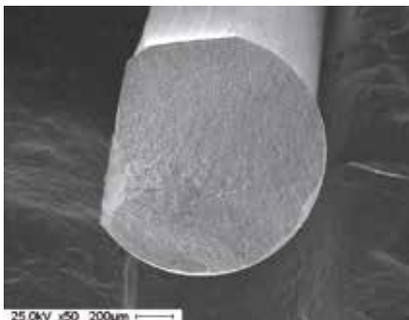
Overview of a spring's fractured surface with a curved forced rupture originating between the inside of the coil and its side surface.
